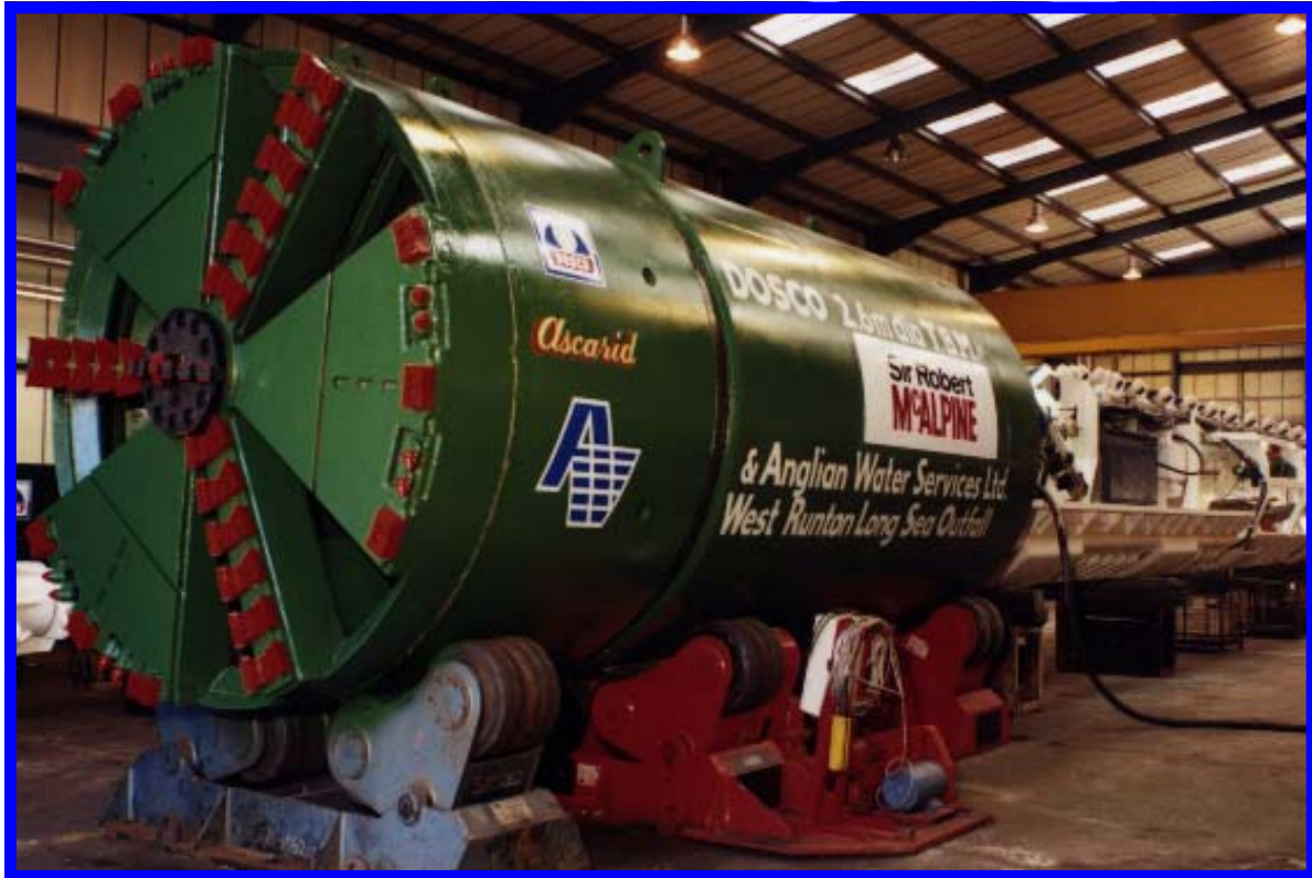
TBM and back-up equipment shown in EPB mode
