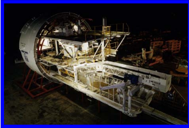
STATION SHIELD triple work decks permit shorter launch tunnels
