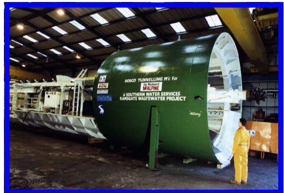
TM1800 back-up system testing
