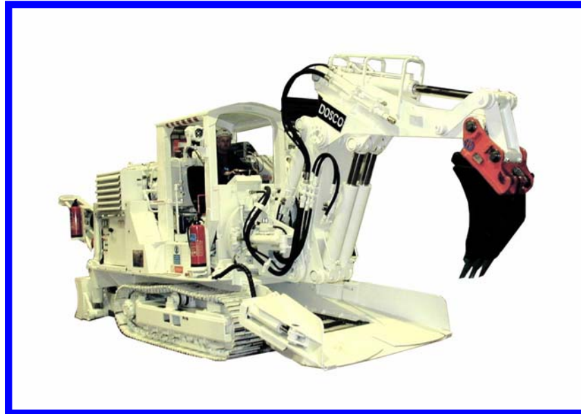
Cross Passage machine shown with rotary backhoe attachment
