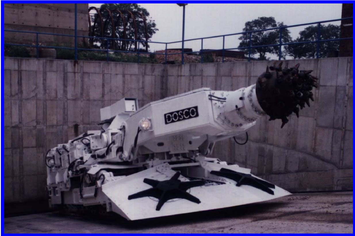
Mk 3 on 1 in 4 incline test ramp
